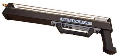
Using a long thin needle the electric power consumption of the resistograph drilling device is measured and recorded. The resistance data gathered provides a high linear correlation between the measured values and the density of the penetrated wood.
