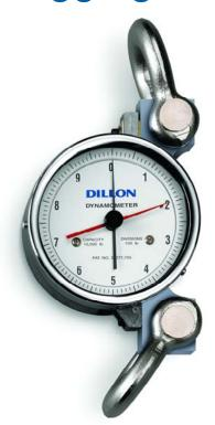
When the wire gets larger, it is more important to follow the sag charts closely. A more detailed sag chart can be provided by engineering that will have sag in inches, pounds and wave time. One of the easiest ways to sag larger conductor is to use the pounds of tension provided and a dynamometer.
