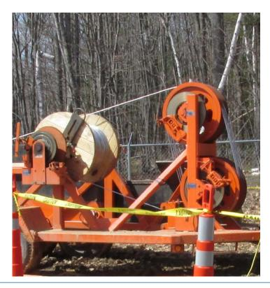
Some are equipped with one brake just on the reel while others have brakes on the reel plus a Schematic (Bull Wheels) with brakes.
